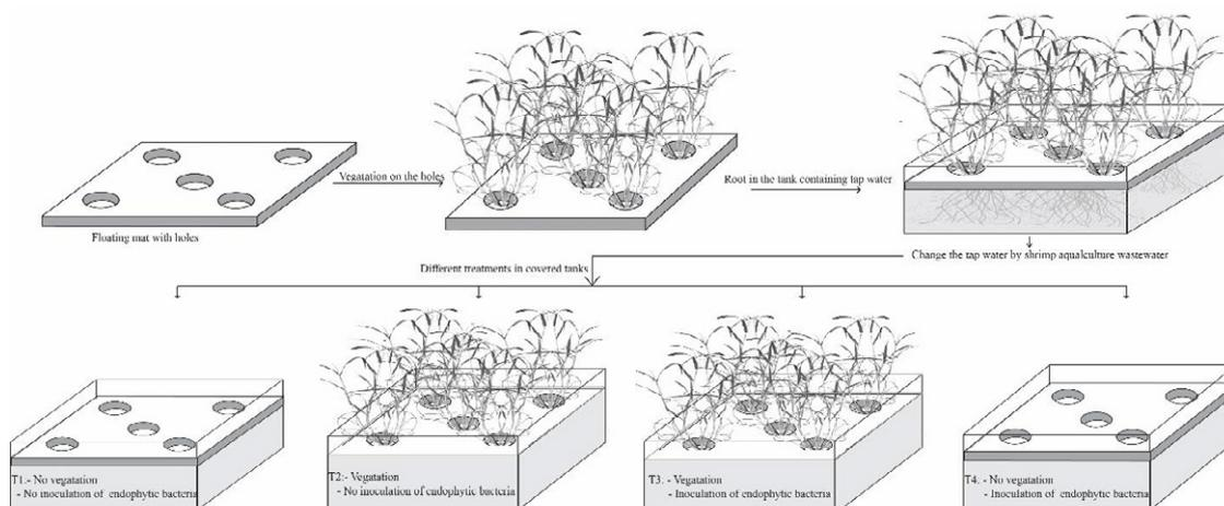
**Fig. 1** Different components of floating treatments wetlands and experimental setup
